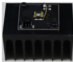
Picture 11. Fins facing down (This orientation obstructs the air flow)
